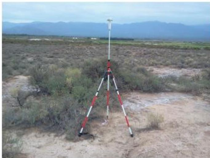
**Figura 1: Receptor GPS, Novatel TechGeo GTRA BT**
