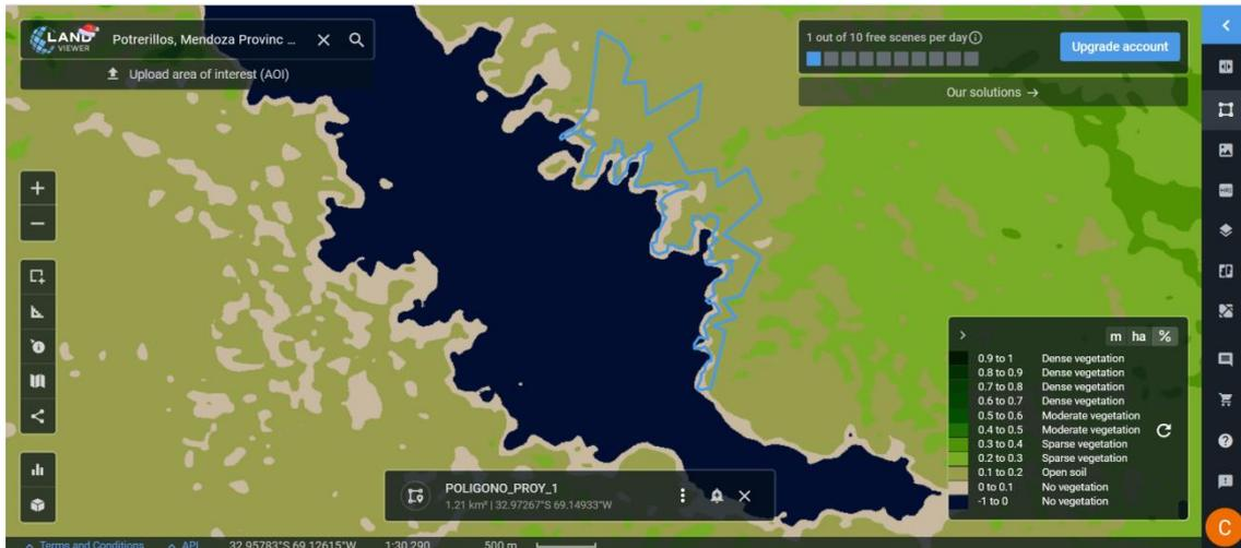
FIGURA 20: VALORES DE NDVI EN EL ÁREA DEL PROYECTO. FUENTE: [https://eos.com/landviewer/?LAT=-32.97774&LNG=-69.15224&z=14&MENUITEM=MYAOI&ID=CBERS\\_4\\_AWFI\\_20241230\\_172\\_135\\_L4&B=NIR,RED&COLORMAP=NDVI\\_V2&EXPRESSION=\(BAND16-BAND15\)%2F\(BAND16%2BBAND15\)&ANTI](https://eos.com/landviewer/?LAT=-32.97774&LNG=-69.15224&z=14&MENUITEM=MYAOI&ID=CBERS_4_AWFI_20241230_172_135_L4&B=NIR,RED&COLORMAP=NDVI_V2&EXPRESSION=(BAND16-BAND15)%2F(BAND16%2BBAND15)&ANTI)
